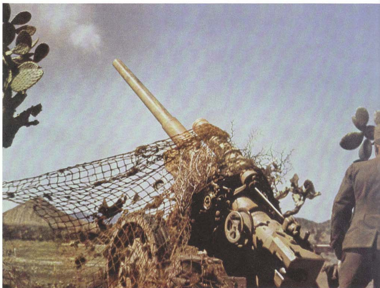
A German 10cm Kanone 18 medium field artillery piece in action in Tunisia. It was really a bit too heavy to be towed by horses, and its small shell weight (15.4kg) was disappointing. It was eventually relegated to coastal artillery. (IWM — TR 152)
