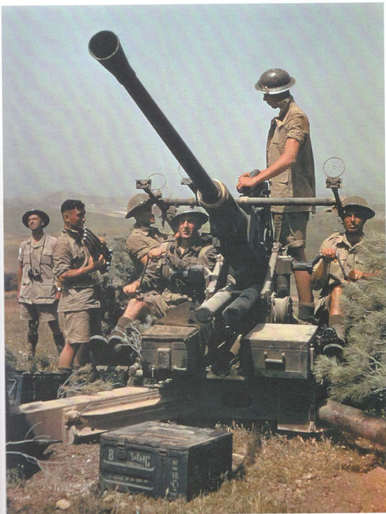
A Bofors light anti-aircraft gun crew in action on the Goubellat Plain near Tunis, May 1943. The Swedish-designed Bofors 40mm LAA gun was probably the best and most widely used of all LAA guns of the war. It was built under licence in the UK. (IWM — 920)
