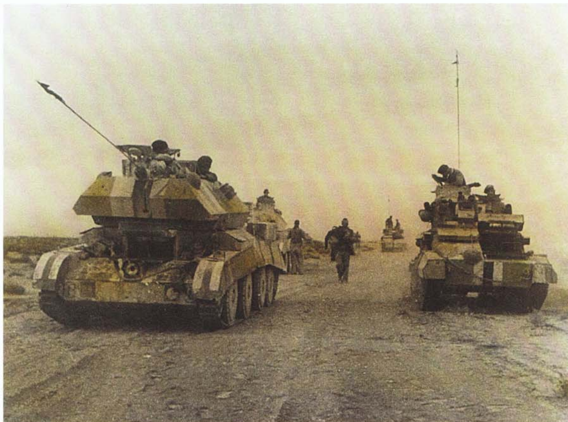
A group of British cruisers and light tanks, all with very prominent white/red/white recognition bands. The light tanks are Vickers Light Mk VI and the cruisers (A13 Mk IIs). Both tanks were fast, but thinly armoured and undergunned. (Author's Collection)
