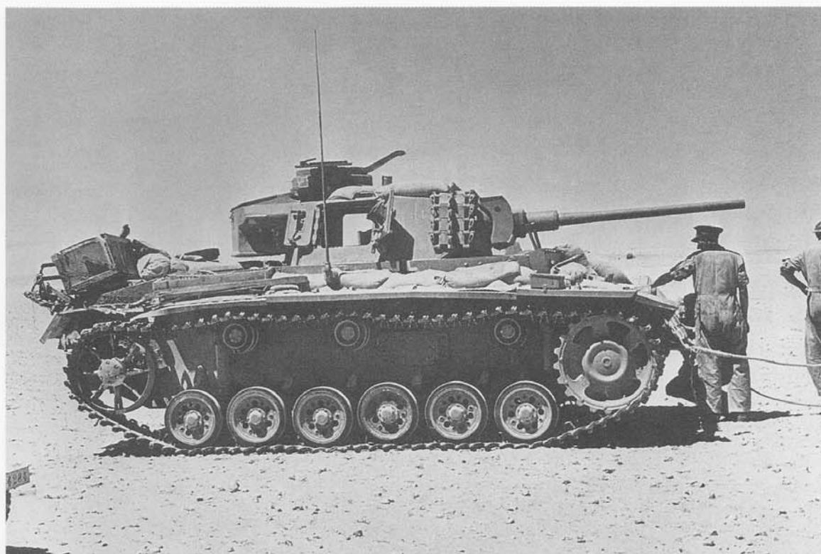
A prize capture. This PzKpfw III Ausf J was known as a 'Special' because its usual 5cm KwK L/42 gun had been replaced with a long-barrelled 5cm KwK 39 L/60, which gave it far greater range and hitting power. (IWM – BM 18476)
