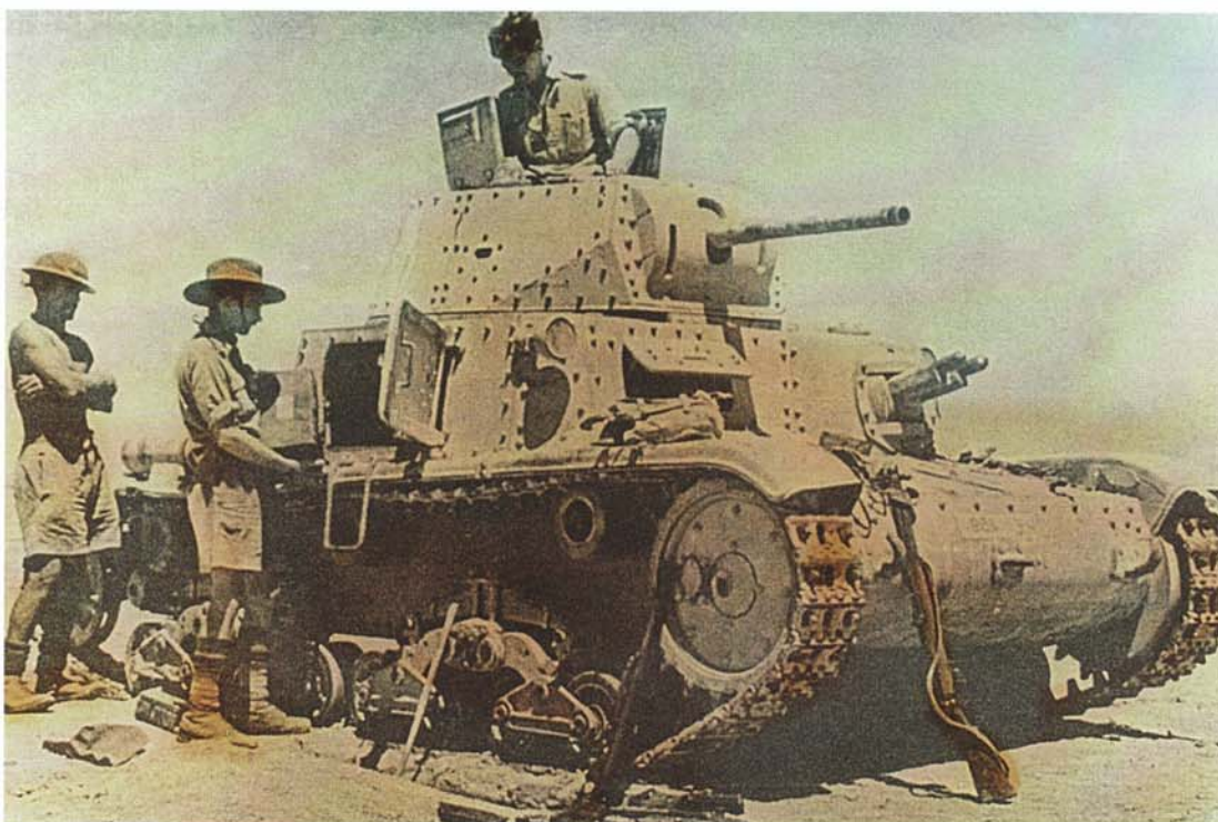
Three British soldiers inspect a knocked-out Italian M13/40 medium tank which had a 47mm gun and weighed 14 tons. It was the best Italian tank to be used in action. (Author's Collection)
